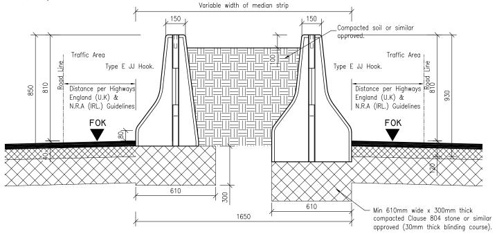
Foundation min dimensions to be min 610mm wide x 300mm deep under each of the concrete barriers. Clause 804 stone or similar approved. 30mm thick blinding course. To be used as a bearing surface for single—sided concrete crash barriers.
